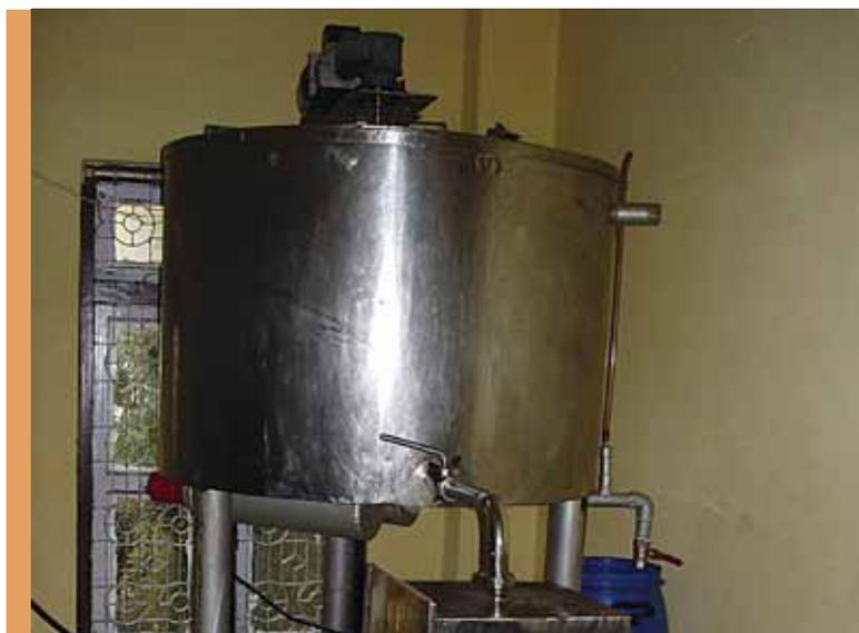
*Processing unit for filtration and moisture removal*
