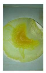
Fig. 1: The wax removed by the Whatman filter
